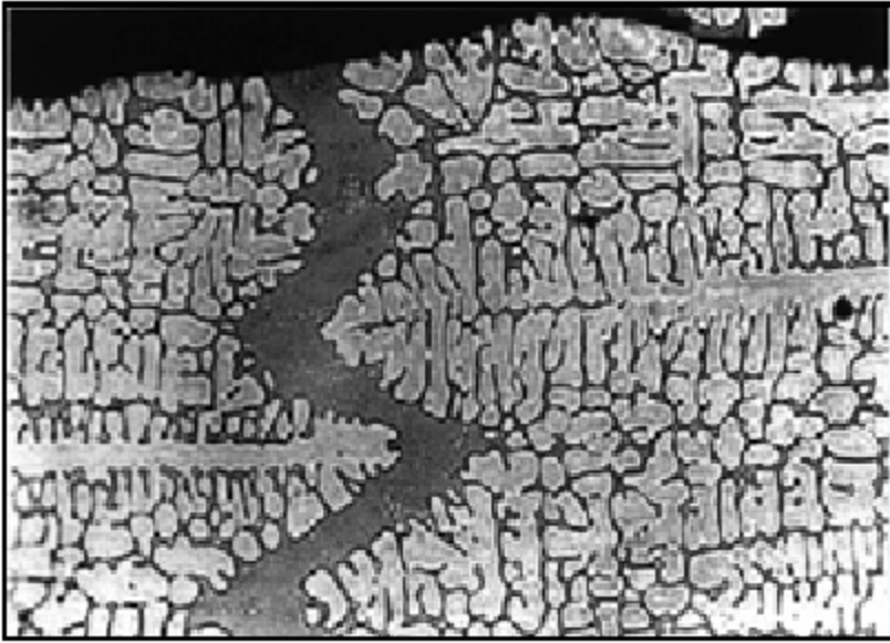
A filled hot tear in an Al-10Cu alloy, not grain refined, cast with 250°C superheat
